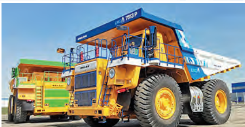
New BELAZ-7513E electric dump truck and world's first 130-tonne BELAZ-7513R truck with gas engine
