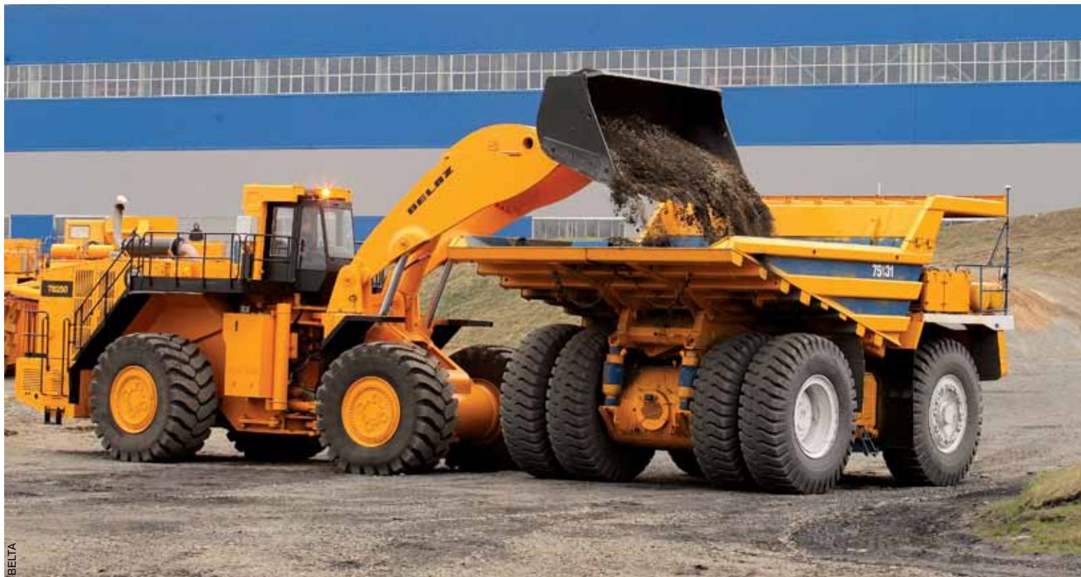
Work by unmanned BelAZ, accompanied by the front-side loader, demonstrated in Zhodino
