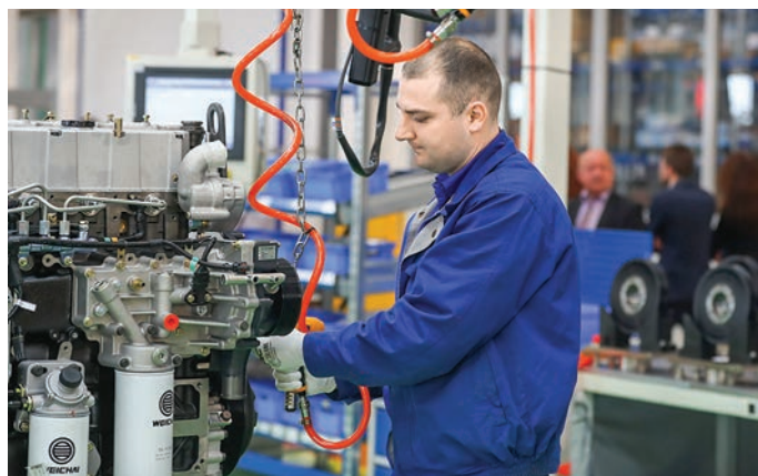
The plant oversees complete knockdown assembly of Euro-5 and Euro-6 engines for trucks, special vehicles and buses. Annual production capacity has reached 10,000 engines, with possible doubling of this figure.
