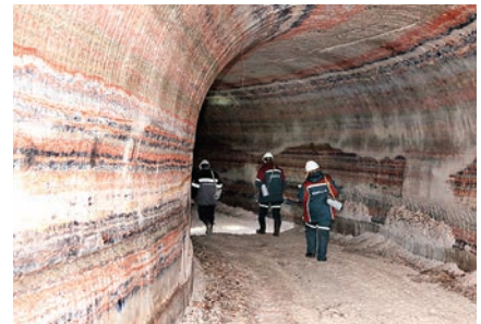
Sylvinite layers create natural patterns on walls of a tunnelling shaft
