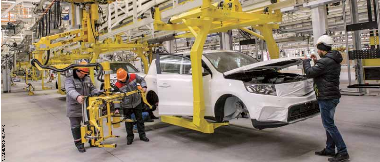
CKD conveyor assembly for Geely vehicles
