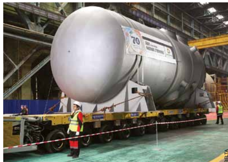
Dispatch of the reactor case for Belarusian NPP
