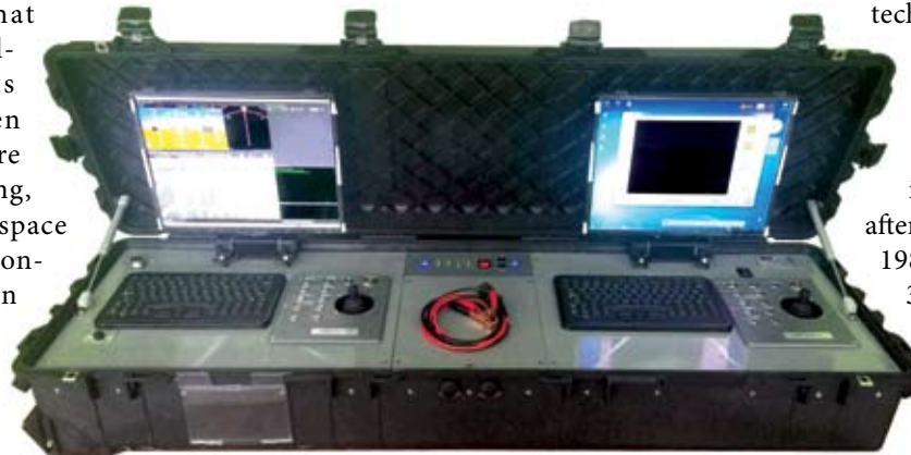
A ground station used to operate unmanned aircraft
